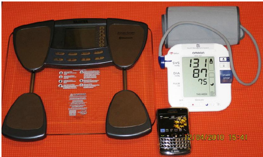
Figure 2. Bluetooth enabled BlackBerry, Tanita Weighing Scale and Omron Blood Pressure Monitor used for Personal Health Data Capture and wireless, automated Data Entry into Personal Health Record (PHR).
